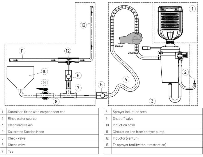
**NOTE**: Flow from the coupler to the check valve should only be downwards. If the venturi is located below the level of the Cleanload Nexus, the check valve may be fitted close to the venturi.
