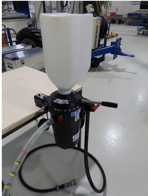
**Filling system for plant protection products Hypro "Cleanload Nexus"**
