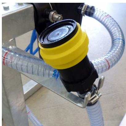
*Fig. 4: The 1" suction hose can be coupled to the plant protection device via the suction connection without dripping.*
