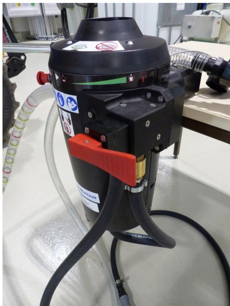
*Fig. 2: The closed container is held by the system and sealed tightly. By turning the dosing handle, the PPP can be sucked in more or less quickly.*
