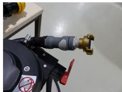
*Fig. 3: The pressurized water connection can be made using the threaded pressure coupling supplied. Appropriate connectors (e.g. GEKA) can be screwed onto the thread (3/4").*
