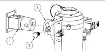
Securely fit the Mounting Point (Ref. 1) to the sprayer, bench, wall or a stand.
