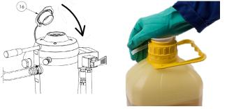
Put the dust cover back on the easyconnect cap for protection during storage.
