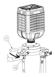
To secure the container to the Cleanload Nexus, move the Operating Handle (Ref. 11) towards the right (anticlockwise) until it passes the closed padlock symbol and stop when it is aligned with the Lock Release Knob (Ref 12) and the droplet image as shown:
