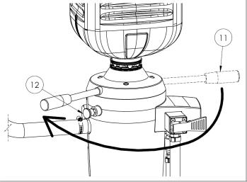
Once the container is empty and clean, move the Operating Handle (Ref. 11) back to the Lock Release Knob (Ref. 12), when you will hear it engage and it will not rotate any further.
