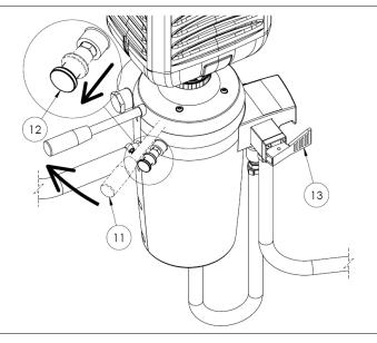
The container can now be released by pulling the Lock Release Knob (Ref. 12) and at the same time moving the Operating Handle (Ref. 11) to the left.
