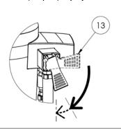
**NOTE**: The Operating Handle (Ref. 11) must be at the correct rinse position (fully to the right at position A), If the handle is not aligned correctly the Rinse Water Lever (Ref. 13) will rotate partially but it will not be possible to raise it or operate rinse.
