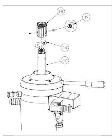
Using a T10 Torque driver, remove the 2 screws (Ref. 19) holding the Probe Head (Ref. 18) to the probe assembly (Ref. 17).
