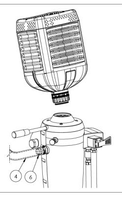
Invert the container and place it onto the Cleanload Nexus as shown, The flange on the easyconnect cap should locate in place, support the container with one hand.
