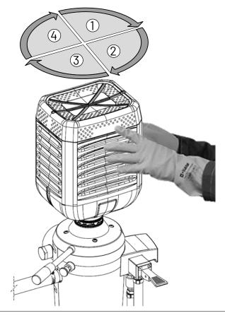
Activate rinse for 15-20 seconds then rotate the container 90 degrees to the left (clockwise) and then release the Rinse Water Lever. Repeat 3 more times for a total of 60-80 seconds.
