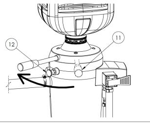
Once the desired quantity has been dispensed, move the Operating Handle (Ref. 11) back to the Lock Release Knob (Ref. 12), when you will hear it engage and it will not rotate any further.
