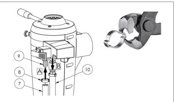
The Rinse Water Supply Hose (Ref. 7) connects to the Rinse Water Supply Hosetail (Ref. 9) at position A.
