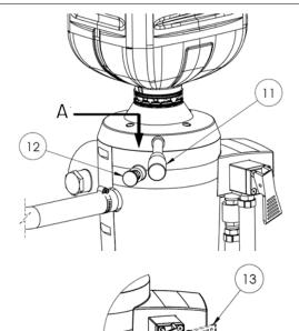
**Note**: If the Operating Handle (Ref. 11) is NOT in the correct rinse position (A), the Rinse Water Lever (Ref. 13) will rotate partially but not engage or operate rinse.
