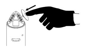
Take the new Umbrella Valves and place the protruding mounts into the corresponding central hole in each valve mounting.
