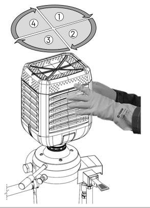
Activate rinse for 10 seconds then rotate the container by 90 degrees to the left (clockwise) and then release the Rinse Water Lever. Repeat 3 more times for a total of 40 seconds for optimum rinsing of the outside of the easyconnect cap and the inside of the Cleanload Nexus.
