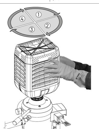
Activate rinse for 10 seconds then rotate the container by 90 degrees to the left (clockwise) and then release the Rinse Water Lever. Repeat 3 more times for a total of 40 seconds for optimum rinsing.
